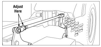
Figure 9. Adjust Lift Rod Timing
